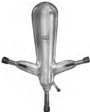
FIG. 344. The tube of the single-phase mercury arc rectifier. The General Electric Co.
